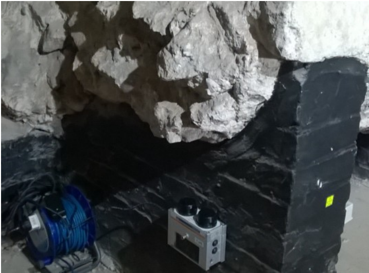
Vibration monitoring of the Roman Wall
